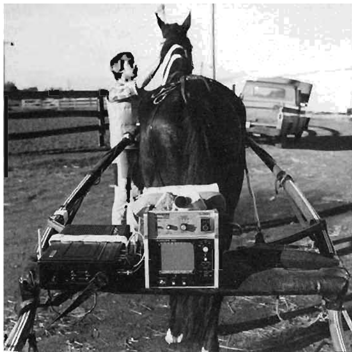
The Exercising Physiology cart at the Franklin County fairgrounds. The cart was developed by Dr. Albert Gabel and others to measure cardiovascular function during exercise. (Veterinary College Files)
